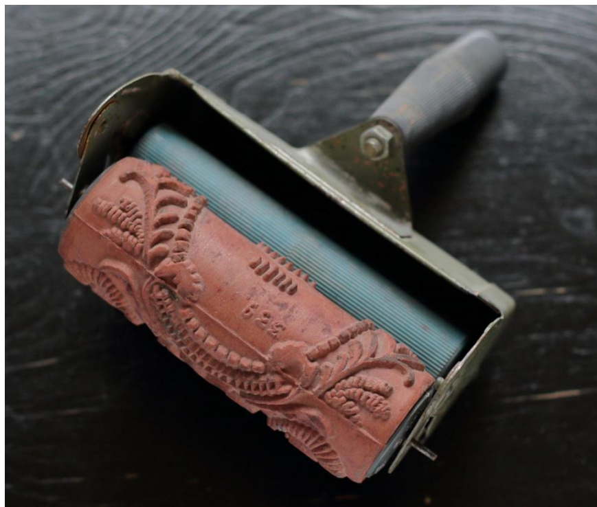
Fig. 10, 11. An old painting roller with pattern. Below: Painting handle with container and rollers distributing the paint.
